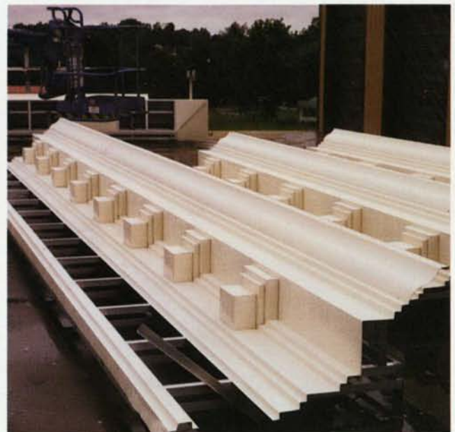
Aluminum Cornice with Aluminum Framework Awaiting Delivery
